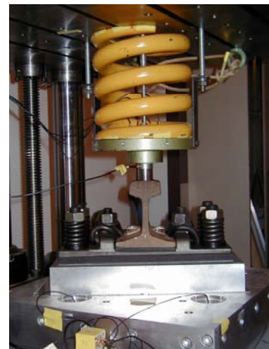
Fig 2: Test rig for dynamic measurements, featuring an installation for rail fastening systems according to ENV 13481-6 [2], (see Fig. 1 for explanation of the functions) [Photo: Rolf J. Diehl, Müller-BBM]
